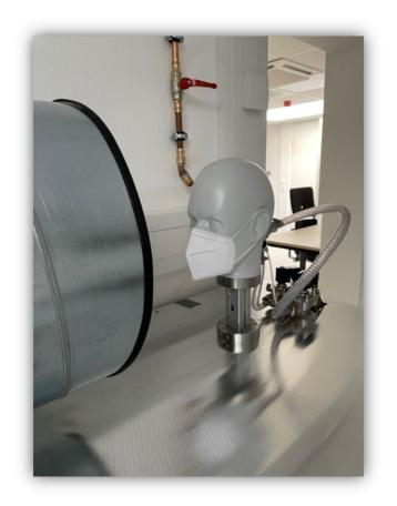
At Hohenstein, standardised test procedures provide information on whether the breathing comfort and filtering performance of everyday masks are adequate.
